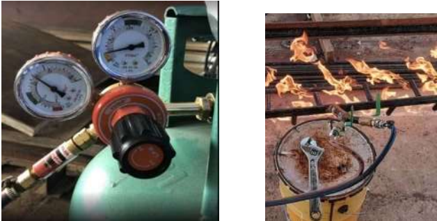
Fig.3 Connect regulator with LPG, O 2 and connect ball valve and quick connect with pipe heat
